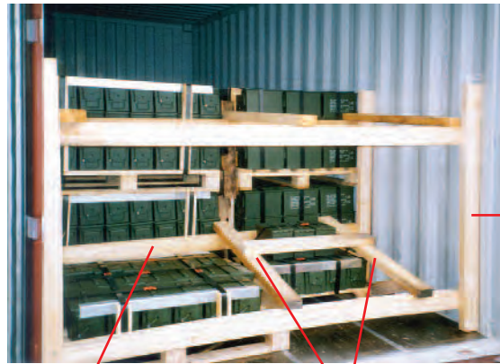
Timber "gate" to restrain cargo and bracing struts running back from gate to rear corner posts to support the gate restrains both upper and lower tiers of cargo.
