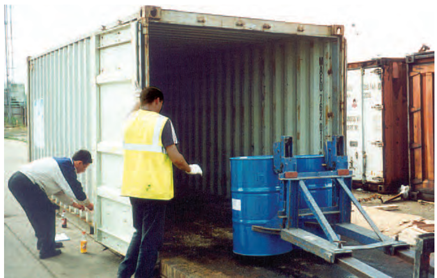
Drums being packed with drum clamps
