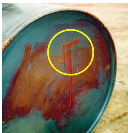
Typical nail-puncture damage Red dye can be seen leaking from a hole made by a nail that was protruding from a broken pallet
